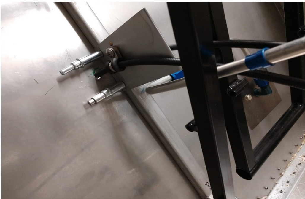
Sonex throttle and mixture cables passing through firewall
