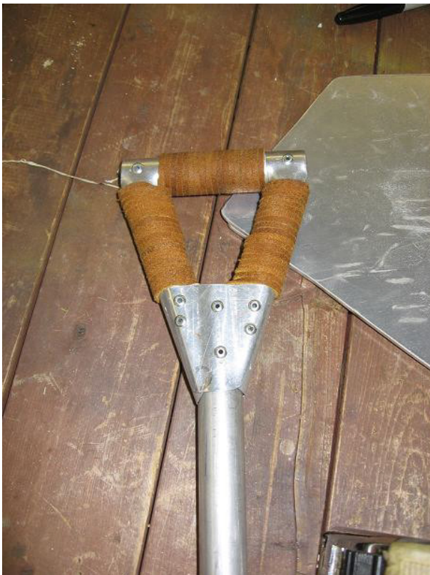
Ben's first work on his Nieuport was to craft this custom control stick grip.
