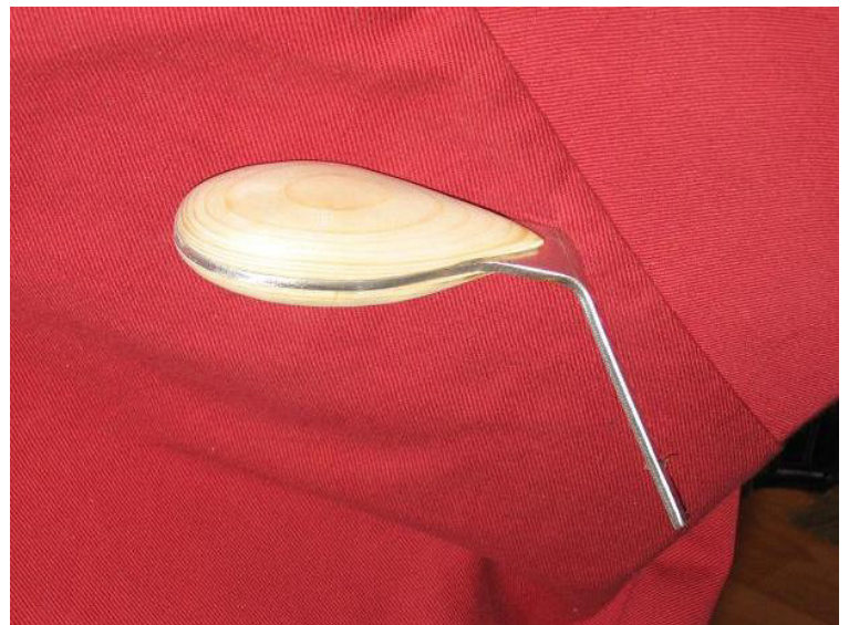
Ben also spent a lot of time researching and making this custom throttle control for his WW I replica biplane.
