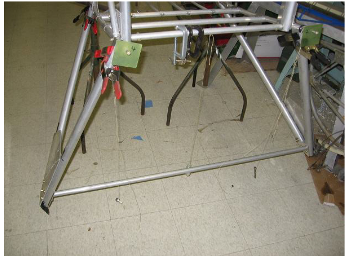
Setting up the landing gear with plumb lines
